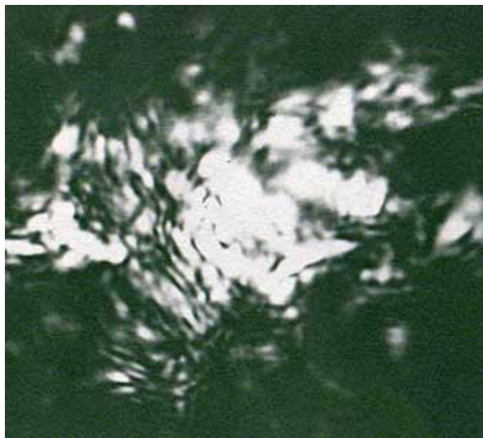
FIGURE 2 – EFFECTS OF SCINTILLATION OF OPTICAL TURBULENCE ON A LASER BEAM AFTER TRAVELLING THROUGH THE ATMOSPHERE
