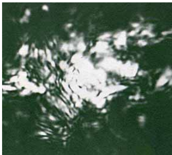
Figure 1 – Effect of Scintillation on an optical beam after traveling through the atmosphere.
