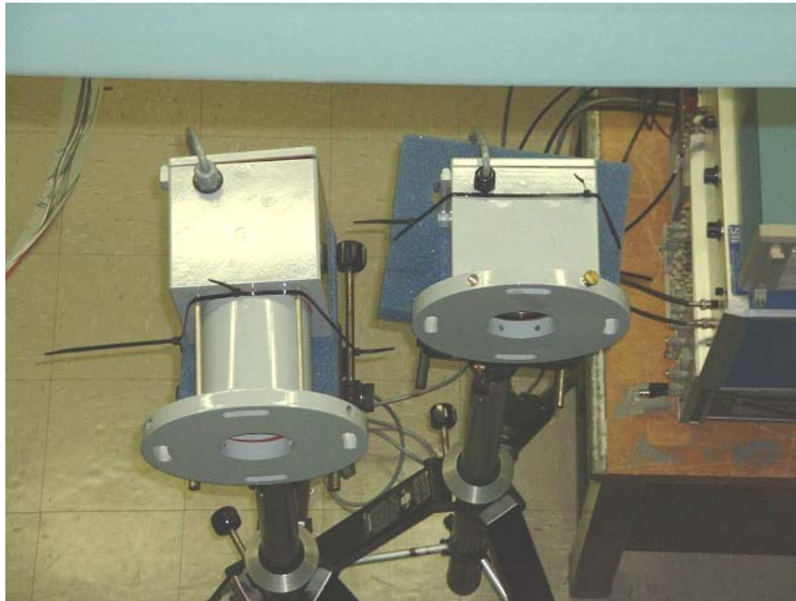
Figure 1. Images of the Optical Scientific, Inc., Optical Flow Sensor System – top view of the receiving optics as installed in the NIST Dual Test Section Wind Tunnel.
