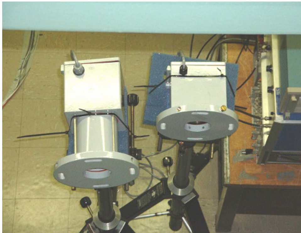
Figure 1. OSi's Optical Flow Sensor Receiver Heads (top view) as installed in the NIST Wind Tunnel.
