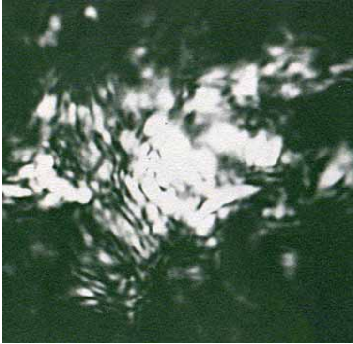
Figure 2 – Effect of Scintillation or Optical Turbulence on a laser after traveling through the atmosphere
